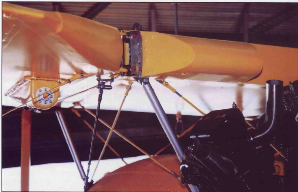
The leading edge light on HD874; details of the port upper and lower wing-fuselage joints. Note the port fuel tank is covered, although the fairings over the centre section struts are not fitted. (All JDK)
