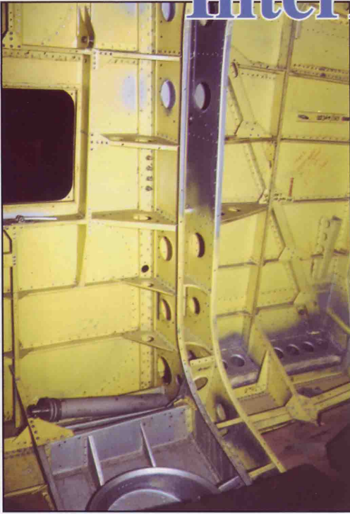
Top left: The hull interior, of G-RNLI, bereft of fittings but showing the double frames around the undercarriage retraction jack position. (JDK)
