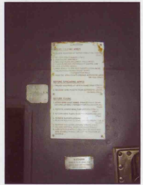
Clockwise from top left: The nose of A2-4 appears to have a side panel that is unique to this machine. (JDK/RMW) The instruction panel for wing folding, fixed to both sides of the fuselage. (JDK) The lower wing-fuselage join, rigging and strut detail. The mooring bollards and nose hatch surround, all on A2-4 (JDK/RMW) Chartboard in hand, the navigator prepares to board an FAA Walrus 'somewhere at sea' aboard a carrier. (IWM)
