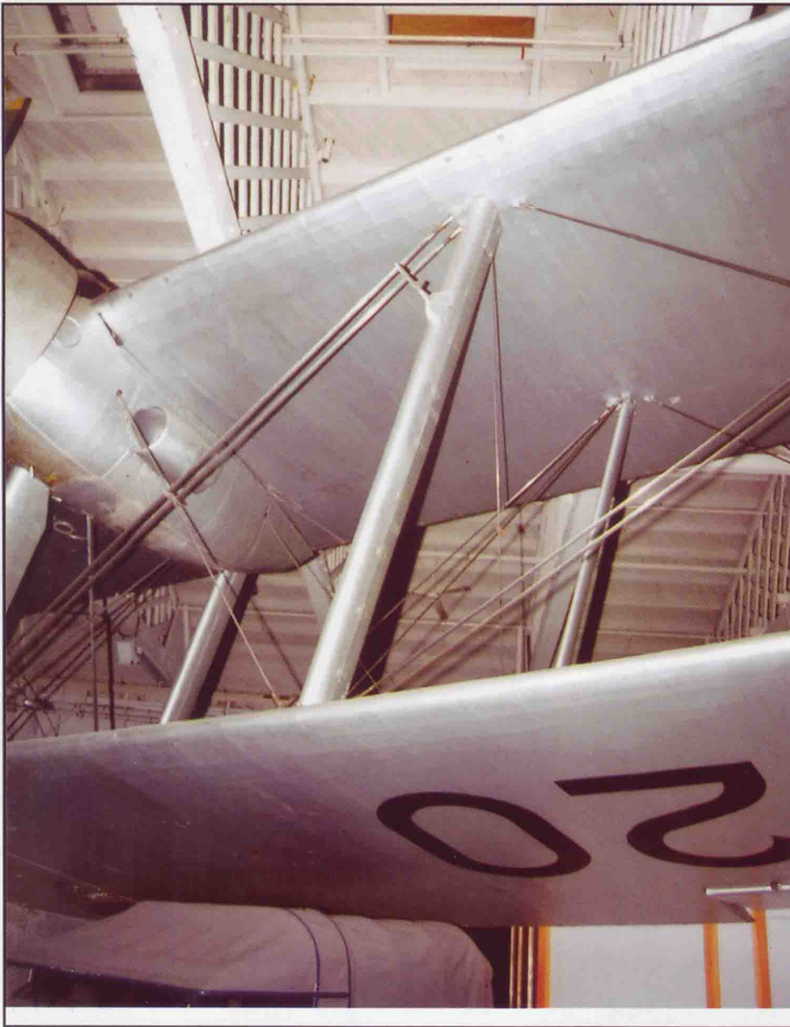
Top left: The port inner bay of 920 with the double flying wires clearly visible.
