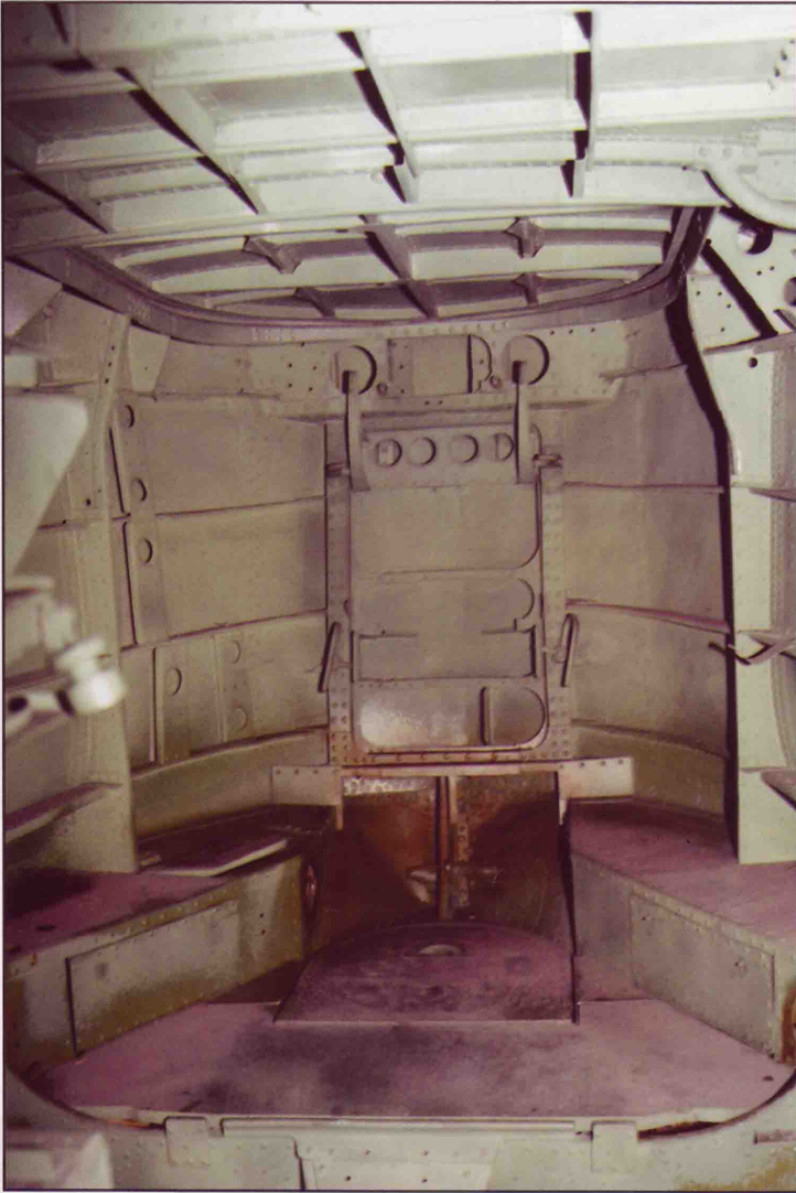
Left: The bow interior, showing internal details of the bomb-aimer's hatch, and the sliding bow hatch above for the bow gunner's use and mooring. All equipment fitted here is, sadly, long gone. Top: Access to the bilges. Bottom right: The crew door from below, showing its complex construction. Bottom left: The interior of the rear fuselage, and walkway to the tail gunner's position.
