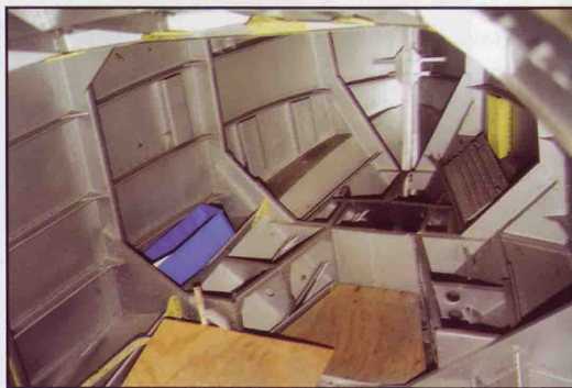
Bottom left: The bow compartment of G-RNLI, showing clearly the frame sections.
