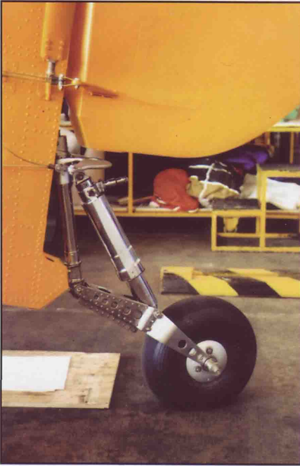
Clockwise from top left: HD874 has the later 'Sea Otter' style tail wheel, without any concession to a water rudder housing, found to be unnecessary. The main wheels on L2301, G-RNLI and HD874 respectively, all showing often-overlooked aspects of this configuration – particularly the small stub which locks into the fuselage side from the main leg. (All JDK)
