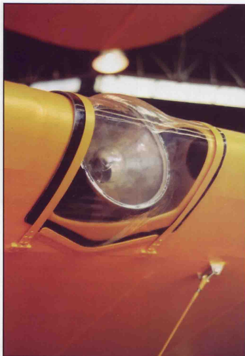
The leading edge light on HD874; details of the port upper and lower wing-fuselage joints. Note the port fuel tank is covered, although the fairings over the centre section struts are not fitted. (All JDK)
