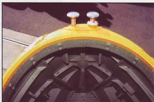
Clockwise from top: The rear fuselage interior of HD874, with the circular drogue case on the right, and the control runs behind that. The nose bollards, and extreme nose interior; the camera mount (when not in use) and the hatch for the camera port. (All JDK)
