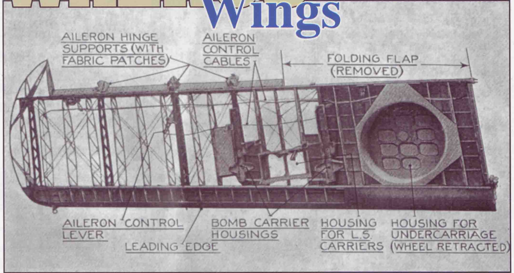
Above: The port lower wing from the manual, showing the large number of fittings required.
