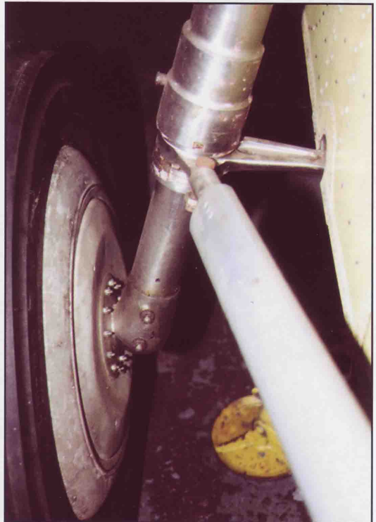
Clockwise from top left: HD874 has the later 'Sea Otter' style tail wheel, without any concession to a water rudder housing, found to be unnecessary. The main wheels on L2301, G-RNLI and HD874 respectively, all showing often-overlooked aspects of this configuration – particularly the small stub which locks into the fuselage side from the main leg. (All JDK)
