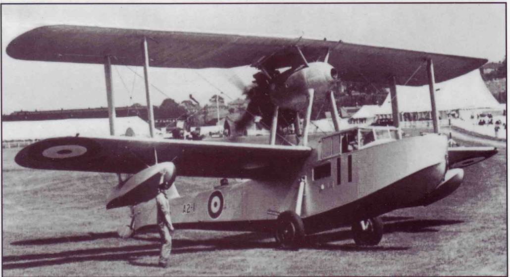
Below: The First Seagull V for the RAAF taxiing at the RAF Hendon Display in 1935, bearing its 'new aircraft number' 11 on the nose. Absent are the inboard jury struts visible on the Walrus Mk.I in the picture above. (JDK collection)
