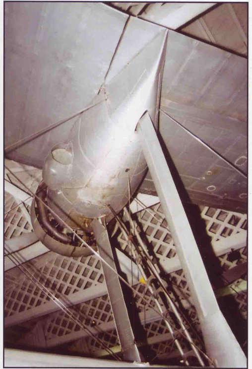
Four views of the nacelle details of 920, as preserved. Engines, props and cowlings are all post-war modifications, but the nacelle struts, wing and fuel tanks are unchanged.
