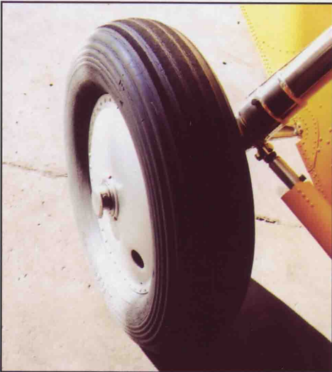
Clockwise from top left: HD874 has the later 'Sea Otter' style tail wheel, without any concession to a water rudder housing, found to be unnecessary. The main wheels on L2301, G-RNLI and HD874 respectively, all showing often-overlooked aspects of this configuration – particularly the small stub which locks into the fuselage side from the main leg. (All JDK)
