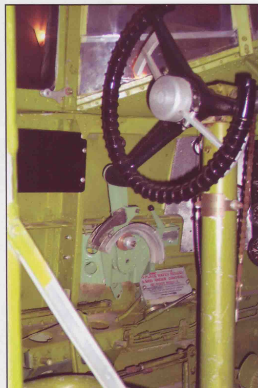
Multiple views of HD874's glazing, with the fall of shot compass fitted inside the erected 'wind-screen'. Note the substantial hinges on the quarterlights. The control column on L2301.
