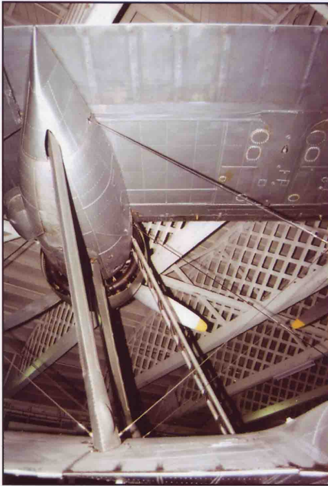
Four views of the nacelle details of 920, as preserved. Engines, props and cowlings are all post-war modifications, but the nacelle struts, wing and fuel tanks are unchanged.
