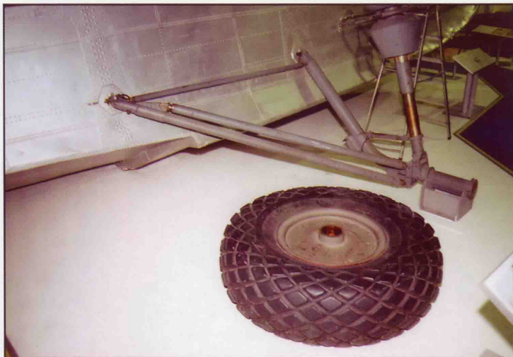
Top: Another view of the starboard beaching gear. Gear varied, and this set is not typical of RAF units, and many Canadian units were also of a different type.
